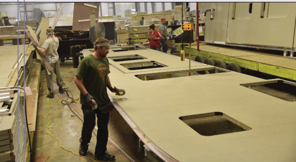
Manufacturing technician Terry Wertz (foreground) preps a wall to apply seam tape. Curtis Fugate (upper left) prepares for the next wall to be routed.
