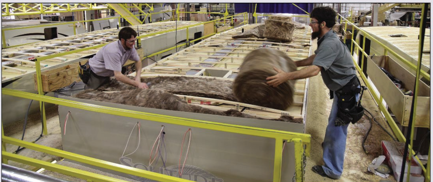
Factory workers roll insulation. Clark says Grand Design has the best workforce in Elkhart County, who buy into the company’s philosophy of high-quality craftsmanship.
